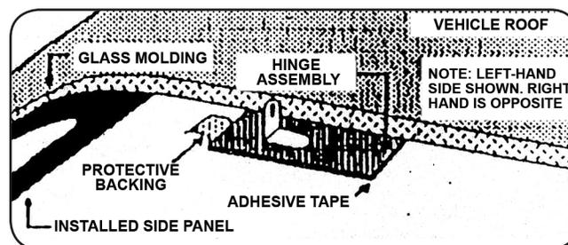
Place the louver on the window with the leading edge of the top slat as close to the window molding as possible and centered side to side. Using a soft lead pencil, mark lightly on the molding the location of the two hinge holes at the top of the louver. Then mark the location of the two tie down studs at the lower outside edges. When all four marks have been made on the molding, take the louver off the window. (On cars without edge molding on the glass, use a crayon and mark the glass-itself).
