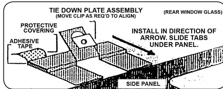
When all attaching hardware has been 'tacked' in place, re-set the louver on the car and fasten the hinges and 1/4 turn tie downs.
